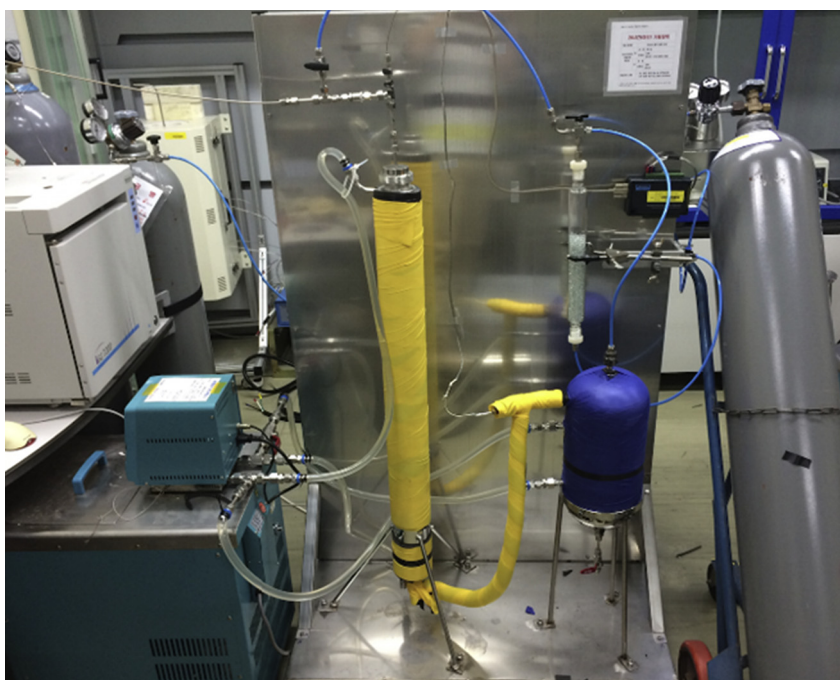
Fig. 5 – Compact xenon adsorption test module with chilled carbon column.
