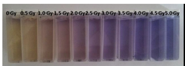
Fig. 5 – The samples after irradiation for 3 hours (30 mM H 2 SO 4 , 0.15 mM Fe(NH 4 ) 2 (SO 4 ) 2 ·6H 2 O, 0.015 mM xylenol orange, and 0.025% glutaraldehyde, 0.075 mM glucose).
