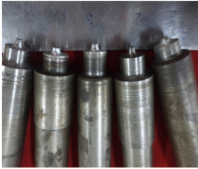
Fig. 2 Fabricated cylindrical threaded FSSW tools
