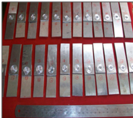
Fig. 4 Fabricated FSSW joints
