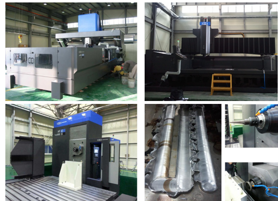
Fig. 10 Example of 2-dimensional hybrid FSW machine at domestic (HWACHEON)
