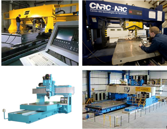
Fig. 6 Example of 2-dimensional FSW machine at oversea
