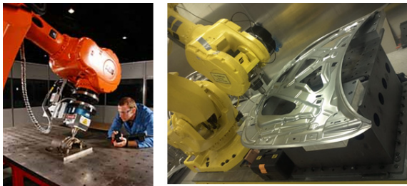
Fig. 7 Example of 3-dimensional FSW machine at oversea
