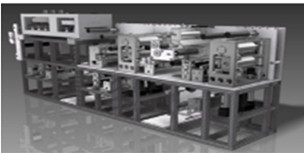
Fig. 1. Design of a roll-to-roll nano micro coating system.
