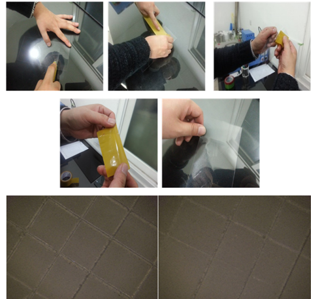
Fig. 8. Adhesive strength test.
