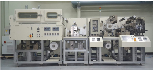
Fig. 2. Practical roll-to-roll nano micro coating system.
