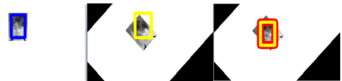
(ii) The meaning of box color for tracking : (Box color - blue: tracking success, yellow: unconfidence, red: detection success)
