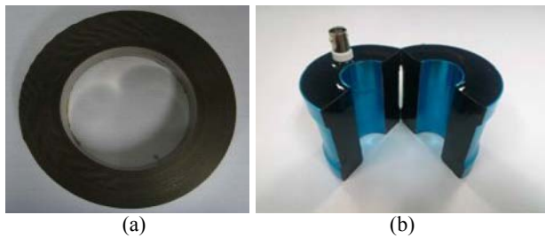
Figure 3: (a) Ferrite magnetic material for an inductive coupling unit, (b) fabricated inductive coupling unit
