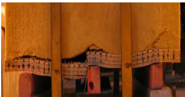
Figure 2: Fracture of plywood in Mark-III
