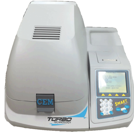
Fig. 2. The appearance of microwave moisture analyzer used in this study.
