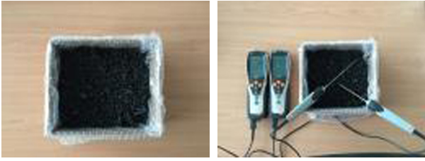
Fig. 4. The experimental apparatus for measuring the temperature change with time at normal temperature and pressure.
