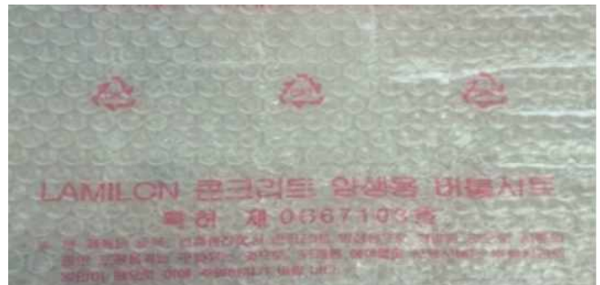
Figure 2. Bubble sheet of ready mixed concrete curing
