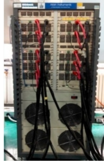
Fig. 6. Arbin BT2000 battery test equipment.
