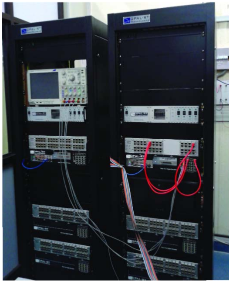
Fig. 3. An image of the OPAL-RT digital simulator.
