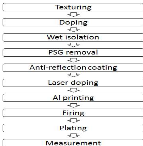
Fig. 1. Fabrication procedure for solar cell.
