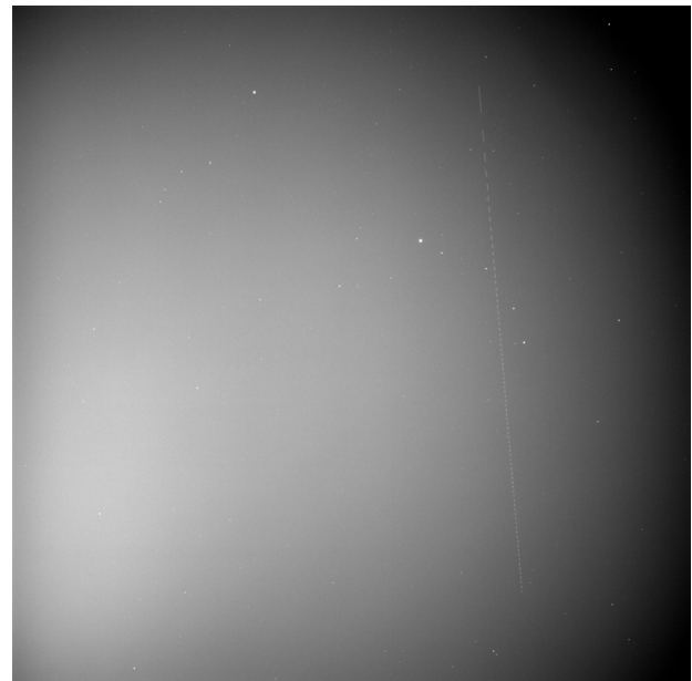
Fig. 8. An optical image of a satellite trajectory taken by the OWL-Net Station in Mongolia. The indistinct dotted line shows a satellite trajectory by a chopper like a electric fan.
