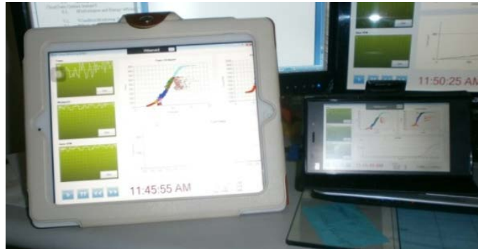
Fig. 11. Instances of the WF CMS accessed remotely from an iOS and Android device.
