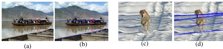
Fig. 8. Examples of linear perspective error: (a) and (c) are input images whereas (b) and (d) show the detected lines displayed in blue, which resulted in misclassification of the vanishing point.
