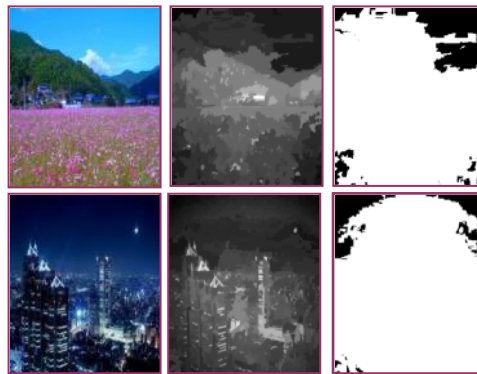
Fig. 12. Examples of scenery images to the left with their corresponding salient maps in the middle, and their binarized salient maps to the right. The ratio defined as the number of white pixels relative to the black ones is used to classify the presence of salient content. In the right figures, the size of the white region is larger than that of the black region, which indicates that no salient object is detected.
