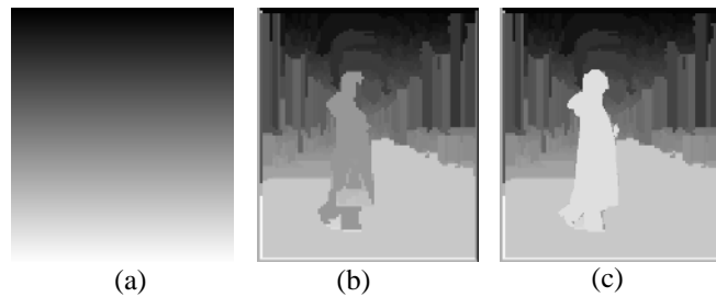
Fig. 6. Examples of (a) type 3 depth gradient, (b) initial depth map, and (c) refined depth map.
