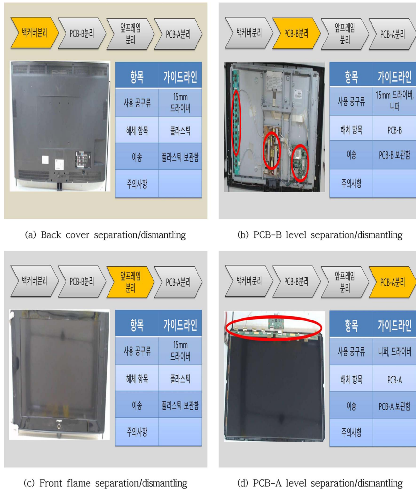
Fig. 1. Separation/dismantling processes of waste LCDs.
