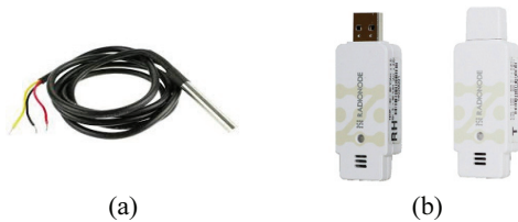
Fig. 3 Sensor for multi-refrigeration system: (a) Refrigerator temperature sensor, (b) Indoor and outdoor temperature and humidity sensor
