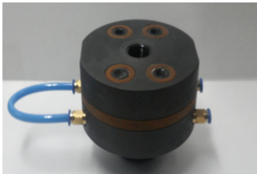
Fig. 3 Insulation apparatus for DCPD.
