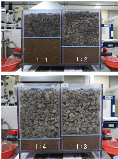
Fig. 1. Experiment model due to ratio of recycle aggregates and ground layer
