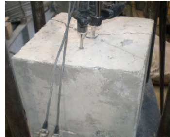
Fig. 3. Failure pattern of specimen
