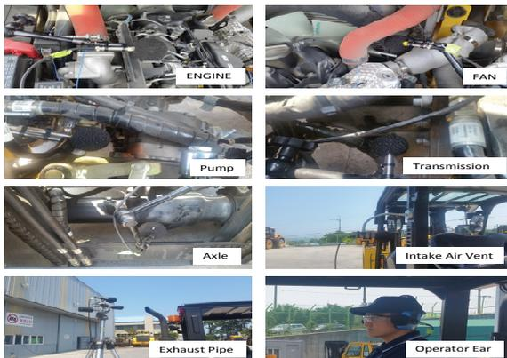
Fig. 1 Measurement position of the noise
