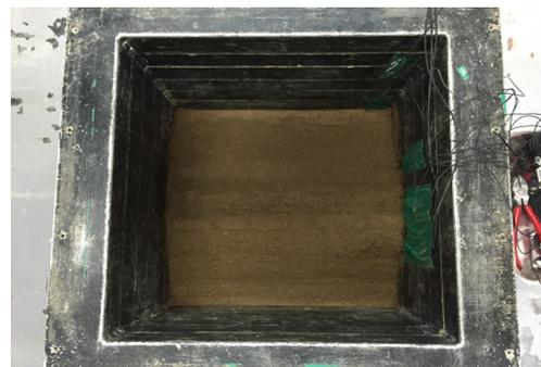
(b) Model reservoir constructed
