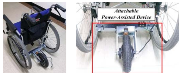
(a) Configuration of PAW (b) Backside of Wheelchair Fig. 11. Configuration of wheelchair.
