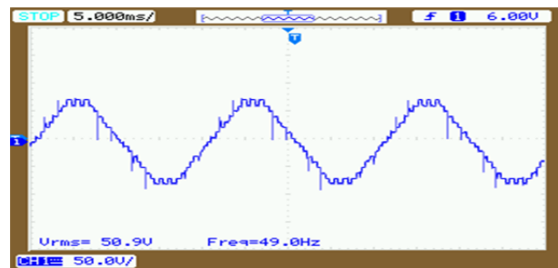
Fig. 16. Experimental output voltage waveform for 100 W load.
