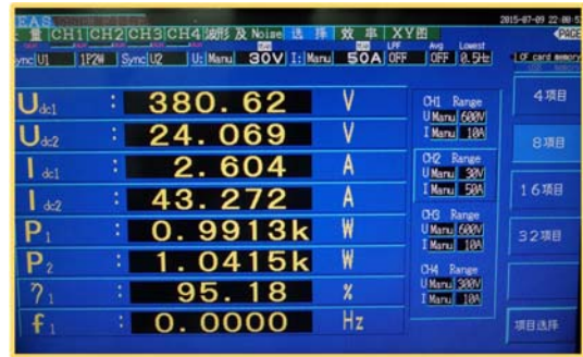
Fig. 13. The measured data of the proposed converter under a full-load condition.
