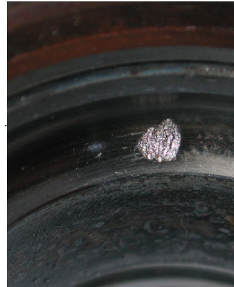
Fig. 5 Fatigue spalling in bearing raceway surface (1)
