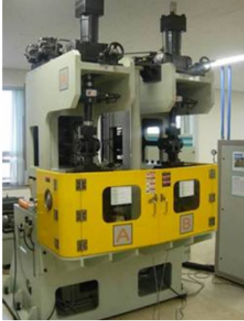
Fig. 3 Automotive wheel bearing life tester (13)
