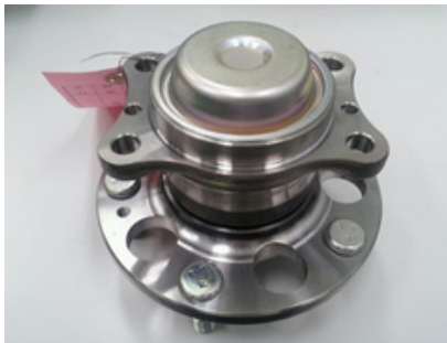
Fig. 4 Gen.3 Automotive wheel bearing (13)
