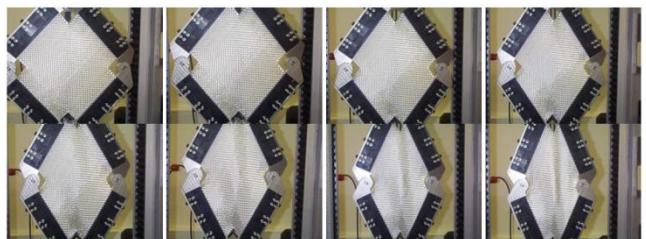
Fig. 6 Picture frame test for the fabric composite[8]
