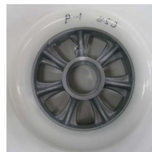
Fig. 11. Fracture of plastic wheel (45 J impact)
