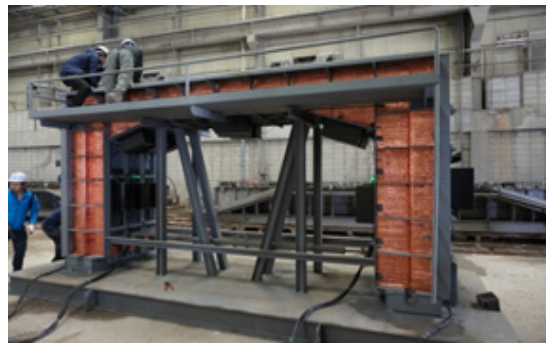
Fig. 2. PC BOX Form for Microwave Heat Curing
