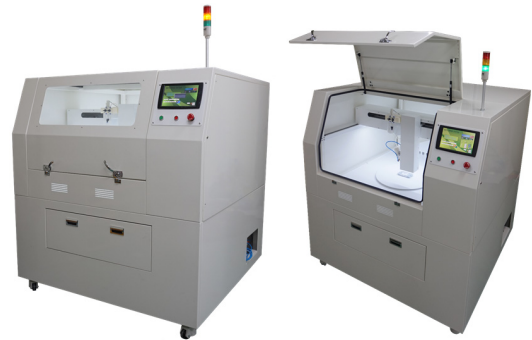
Fig. 2. 3D auto surface preparation system
