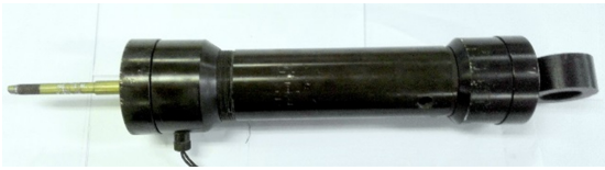
Fig. 3 Photograph of MR damper
