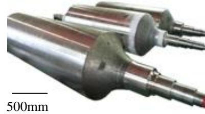
Fig. 1 Hearth roll shape used in continuous annealing line[7]
