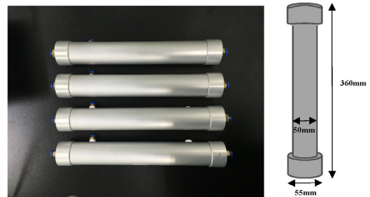
Fig. 2. Picture of the test module and housing for hollow fiber membrane.
