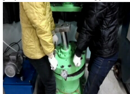
⑤ Dismantling of cover and rod
