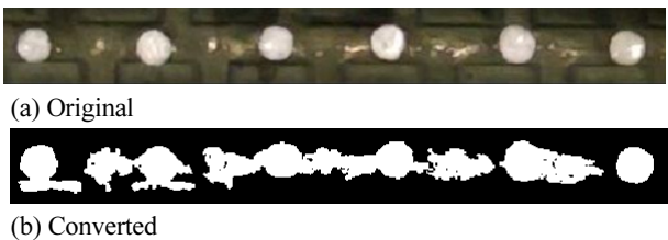
Fig. 3 Inaccurate image processing results due to circumstance and light conditions
