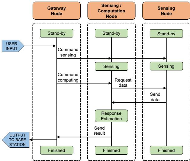
Fig. 4 Flowchart of the response estimation software
