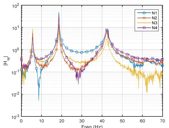
Fig. 6 Magnitude of the estimated frequency response function
