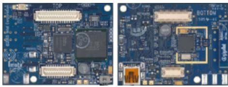
Fig. 1 Imote2 smart sensor platform(left: front, right: back)
