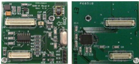
Fig. 2 ISM400 acceleration sensor board(left: front, right: back)
