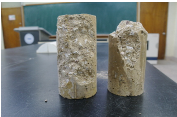
Fig. 12 Compressive strength specimen exposed in fire chamber
