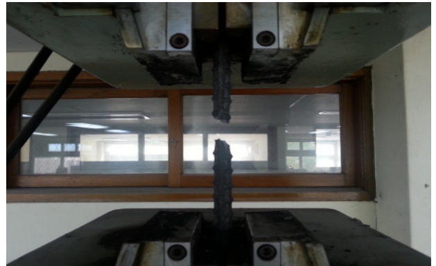
Fig. 21 Test of tensile strength of fire exposed steel bar
