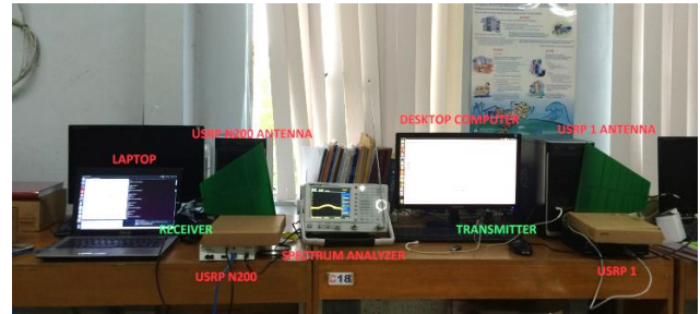
Fig. 3. Experimental setup of the spectrum sensing system of the modified ISDB-T.
