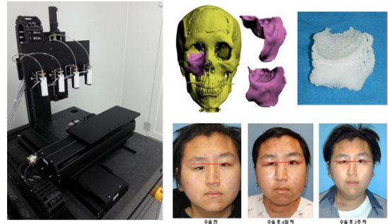
Fig. 5 T&R Biofab's 3D bioprinting system (left) and its application to patient customized facial bone reconstruction
