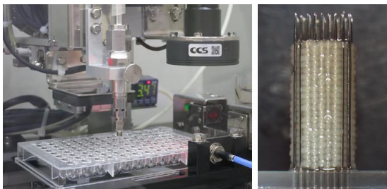
Fig. 4 Cyfuse Biomedical's bio 3D printer, Regenova (left) and 3D printed vessel tissue using skewering cell spheroids onto the needle array (right).
