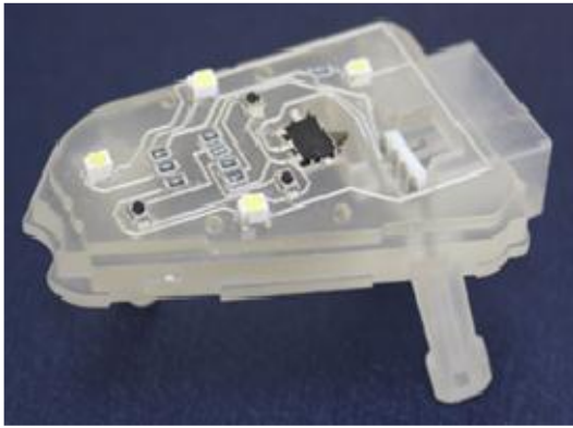
Fig. 8 Fabrication of 3DCD cruise control switch
