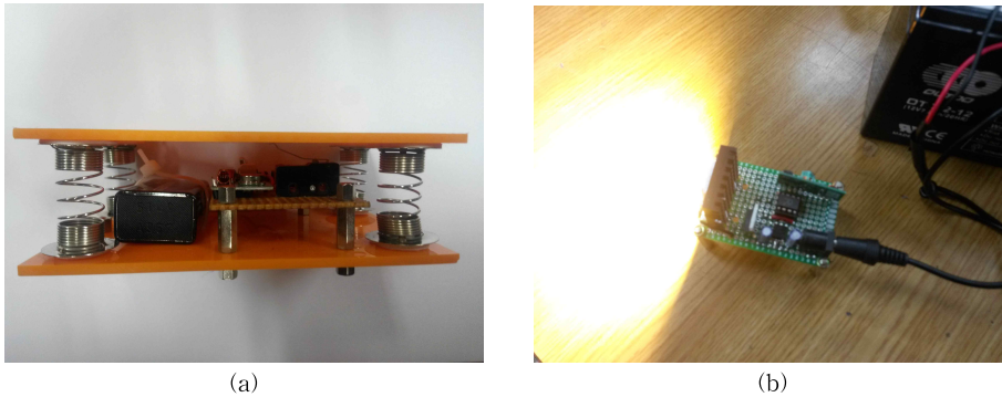
Fig. 6. (a) Approaching sensing module and (b) LED blinkers using RF receiver module.
