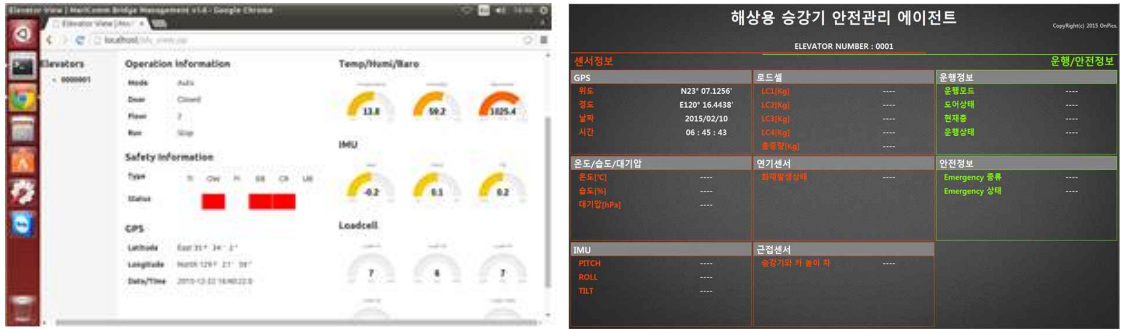
Fig. 5. Agents monitoring device S/W & Marine Elevator Safety Monitoring Server S/W.
