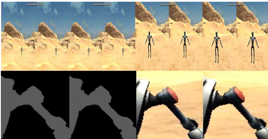
Fig. 11. Testing in a Real Environment. Top : 3D Movie Clip for Robot in the Desert. Bottom Left : Segmented Binary Depth Map. Bottom Right : Inpainting Results.
