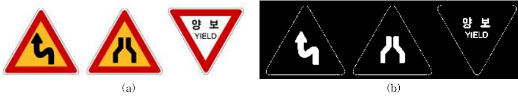
Fig. 4. Comparison between road sign templates and extracted symbols in road sign templates, (a) indicating signs(red, triangle), (b) extracted symbols using edge extraction method.
