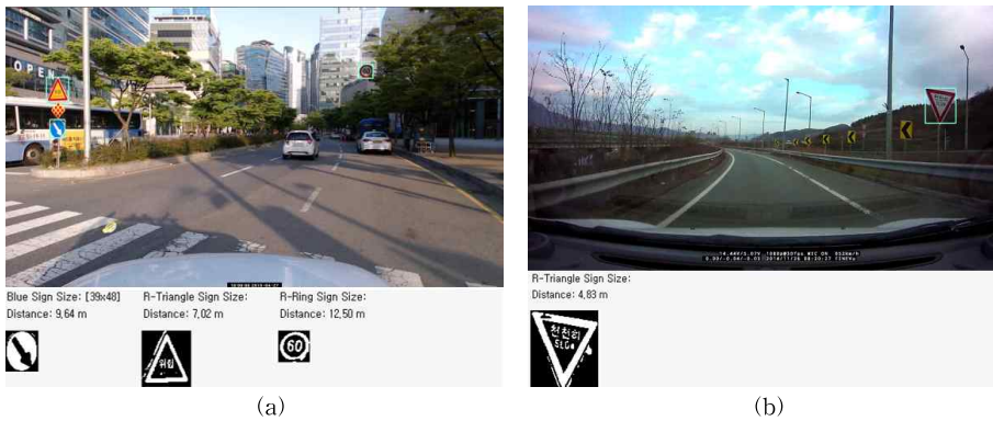
Fig. 7. Test Results for road sign recognition, (a) Busan, (b) National highway between Yeongcheon and Geoncheon.
