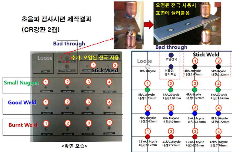
Fig. 8. Standard welding specimens used in this experiments.
