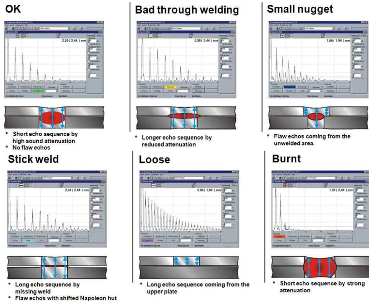
Fig. 6. Characteristics of echo signal according to the results of spot welding.
