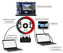
Fig. 2. Simulated driving task diagram
