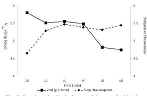
Fig. 3. Steering wheel grip force and degree of subjective sleepiness over time
