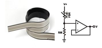
Fig. 1. FSR-408 strip sensor and its schematic
