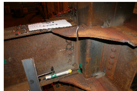
Fig. 13. HBC-3 (failure at upper diaphragm during 0.04rad)
