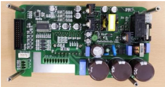
Fig. 5 Board of the designed BLDC motor driver
