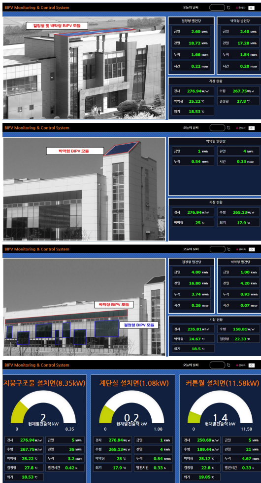
Fig. 11 Window-type and Roof-type BIPV module monitoring system
