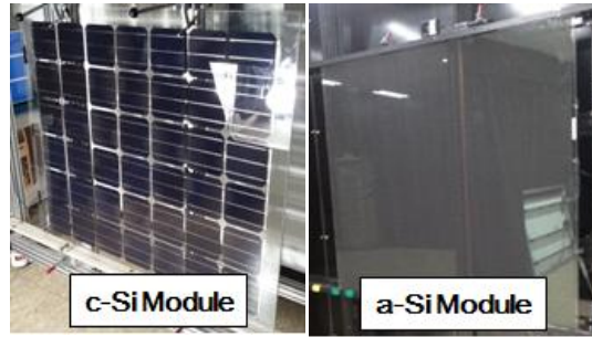
Fig. 4 BIPV module applied to outdoor field test
